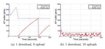
Fig. 4. Histories of buffer size and buffer occupancy with the eBDP algorithm. In (a) there is one download and no upload flows. In (b) there are 1 download and 10 upload flows. 54/6Mbps physical data/basic rates.
